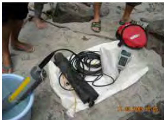
Fig. 5.1. YSI (Yellow Spring Instrument) multipurpose model no. 6600 and TROLL multi-parameter series no. 9500.
