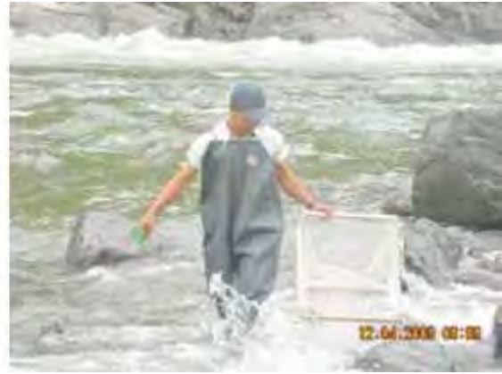
Fig 5.6. Benthos sampling using D-shape kick-net.
