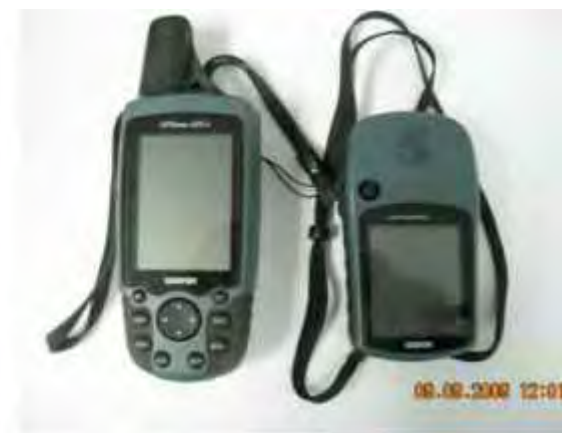
Fig. 5.3. GARMIN GPS models GPSmap 60CSx and etrex-Legend Cx.
