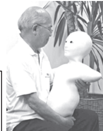
A man communicates with his granddaughter via the new humanoid robot called Telenoid R1 in Osaka, Japan. The robot can robot that can mimic speech and gestures sent to it by video-phone, replicating a distant caller's presence. INTERNET
