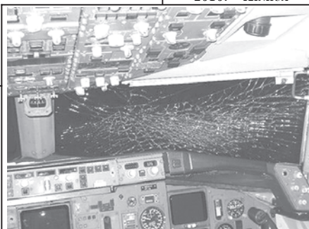
In this image released by the NTSB, heat from electrical arcing in the windshield heater of this American Airlines Boeing 757 shattered the windshield, spraying the flight's first officer with glass while the plane was over the Atlantic Ocean en route to Philadelphia from San Juan, Puerto Rico, on 30 Jan, 2008.—INTERNET
