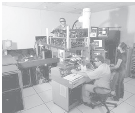
Making adjustments to the dynamic transmission electron microscope. From left: Curtis Brown, Thomas LaGrange and Judy Kim.—INTERNET
