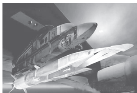
Hypersonic X-51A "Waverider" aircraft produced by the Boeing Company makes a successful test flight on 26 May, 2010. The vehicle flew at five times the speed of sound for about three minutes. Powered by a scramjet engine, X-51A is designed to ride on its own shockwave, furnishing the US Air Force with a long-sought Prompt Global Strike capability. INTERNET
