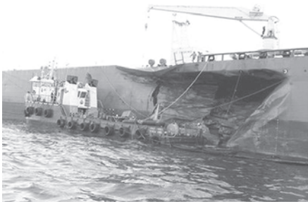
This photo shows a 10-metre gash on the port side of tanker MT Bunga Kelana 3 after colliding before dawn off the east coast of Singapore with bulk carrier MV Waily. Emergency teams have been scrambling to contain thousands of tonnes of crude oil that spilled into waters near one of the world's busiest ports.—INTERNET
