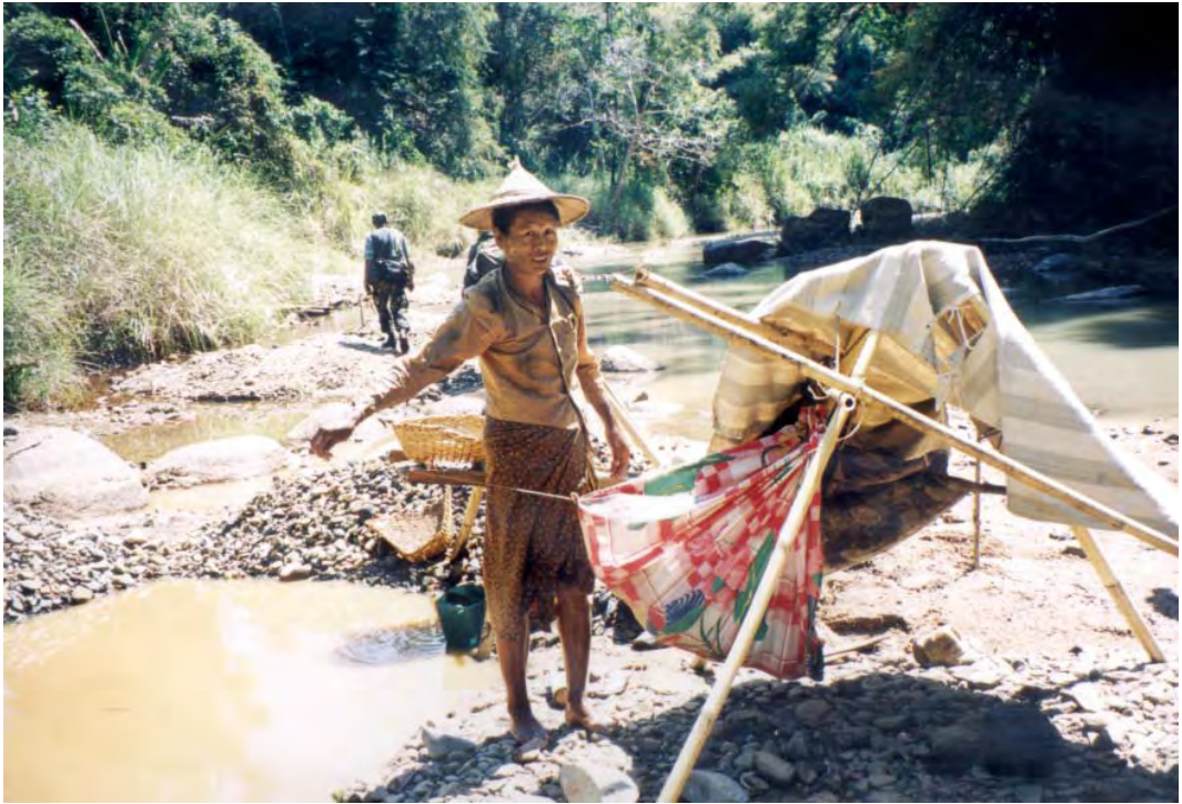
A local villager and his traditional gold-mining apparatus in the dry season. The holes in the riverbed are very shallow.
