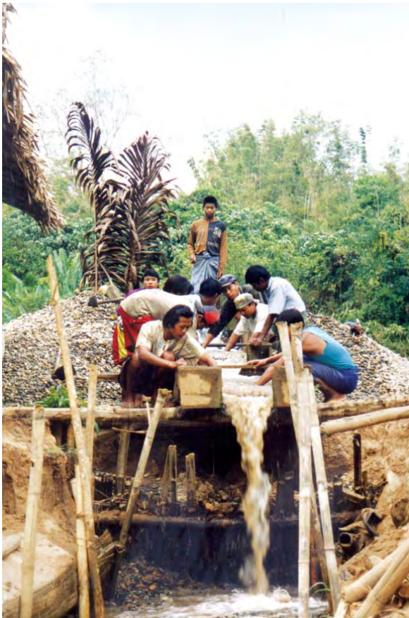
A gold mining sluice in operation
