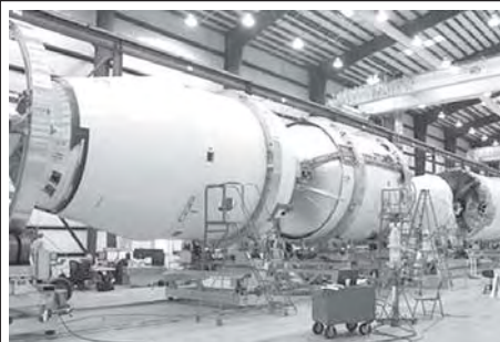
Flight hardware for the inaugural launch of the Falcon 9 rocket undergoes final integration in the hangar at SpaceX's Cape Canaveral launch site in Florida. Components include: Dragon spacecraft qualification unit (left), second stage with Merlin Vacuum engine (centre), first stage with nine Merlin 1C engines (right). INTERNET
