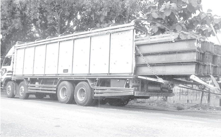
A truck with overload of iron trusses seen on a road.
