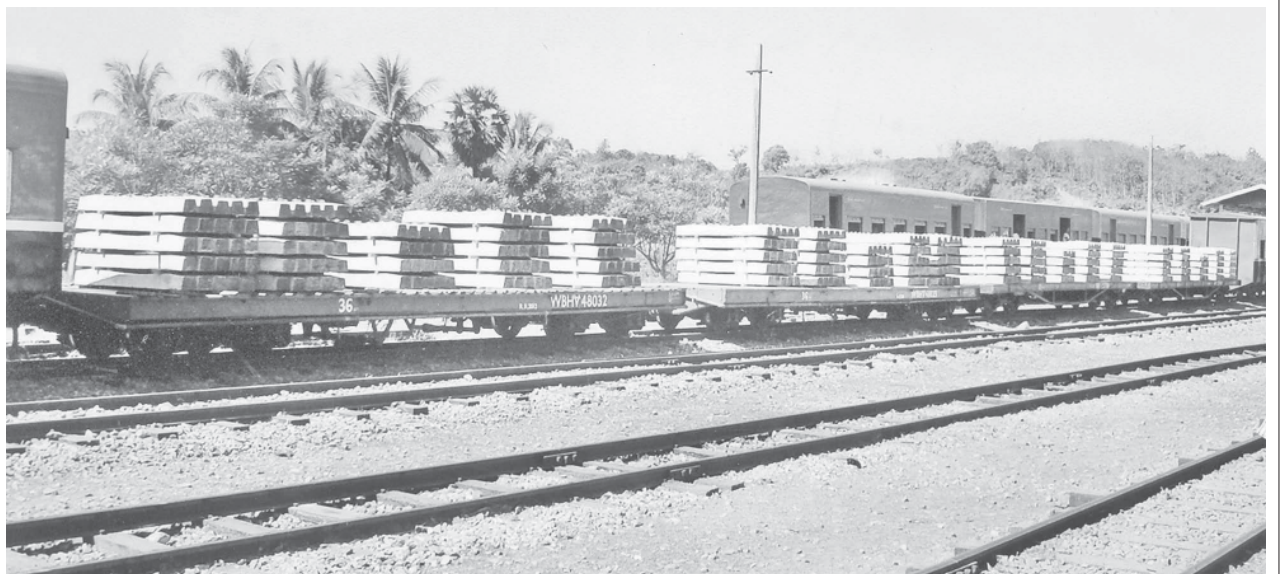
Concrete sleepers from Mottama Factory being transported.
