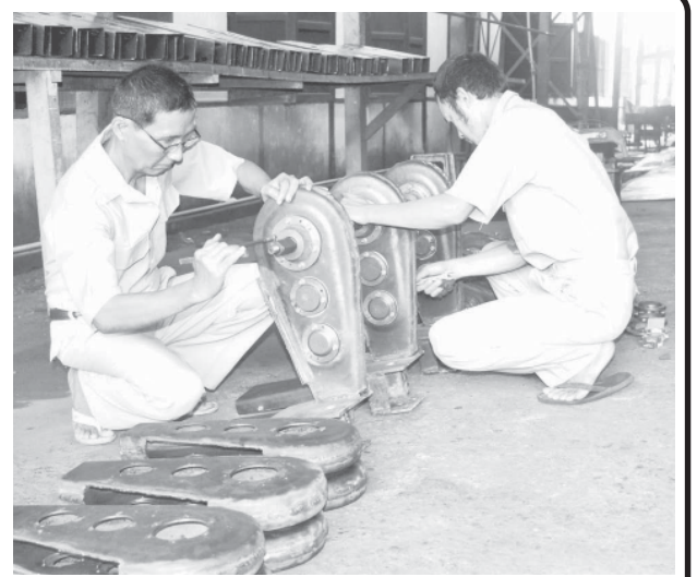
Two workers making gear boxes of power-tillers at No (3) Farm Machinery and Machine Tools Factory in Kyaikkalot, Mingaladon township.
