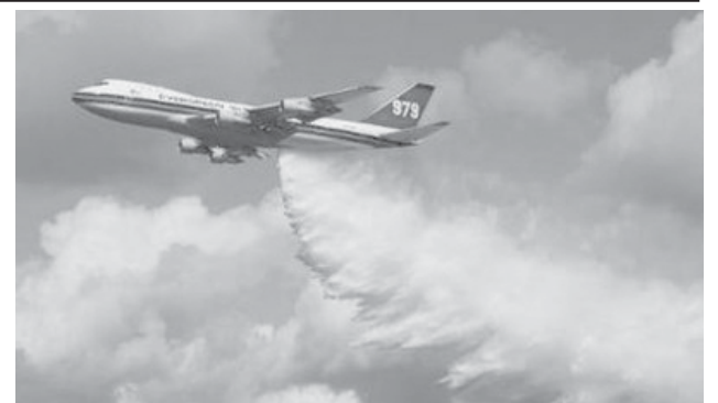
A B-747 Supertanker drops water during a demonstration at the Frankfurt Hahn airport, 100 kilometers (60 miles) west of Frankfurt on 24 July, 2009. The B-747 fire-fighting aircraft is capable of dispersing 20,500 gallons of retardant.—INTERNET
