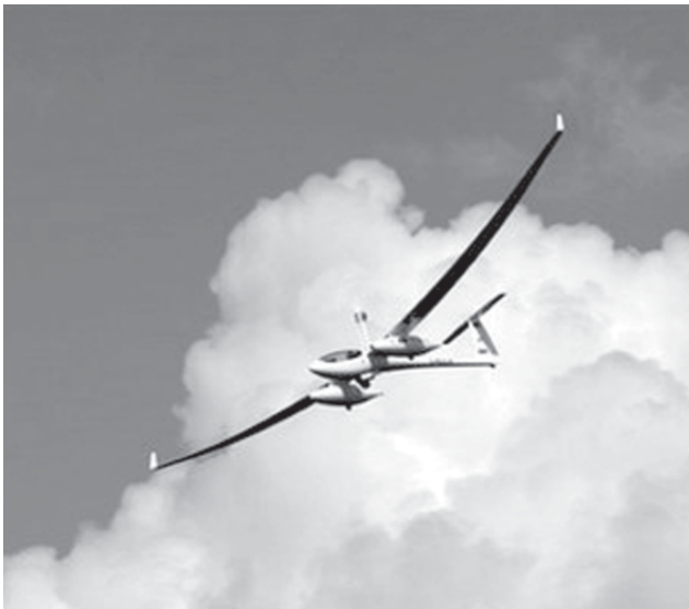
The Antares DLR-H2 flies its madden voyage over the northern German city of Hamburg. The airplane powered by fuel cells was commissioned by the German Aerospace Centre (DLR) with the goal of developing fuel cells for a reliable on-board power supply for wide-body airliners.
