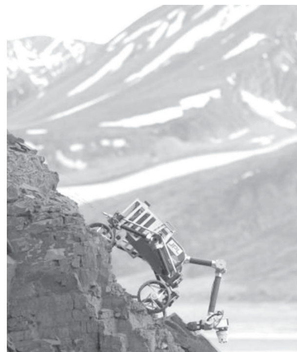
Testing of next generation rovers onboard the Arctic Mars Analogue Svalbard Expedition.
