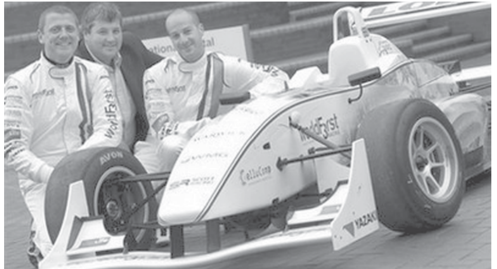
This undated photo made available in London on 5 May, 2009, by the University of Warwick, shows a formula 3 racing car - the WorldFirst Formula 3 racing car - which is powered by chocolate, has a steering wheel made out of plant-based fibres derived from carrots, has bodywork made from potatoes, and can still do 125mph.—INTERNET
