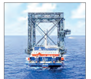
This drone photo taken on 10 July 2026 shows the successful capture of the returned first stage of Long March-10B carrier rocket on a seaborne platform via a net-capture system. PHOTO: XINHUA
