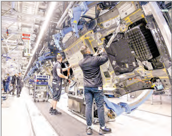
Employees of German car maker Mercedes-Benz work on the bottom side of an EQS passenger car at the 'Factory 56', a completely digitized assembly line, at the Mercedes-Benz manufacturing plant in Sindelfingen, southwestern Germany, on 13 February 2023. PHOTO: AFP
