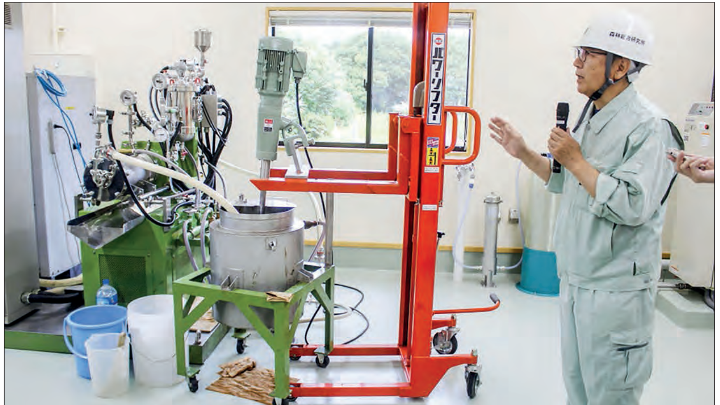
Equipment for pulverizing wood into mash is pictured at the Forestry and Forest Products Research Institute in Tsukuba, Ibaraki Prefecture, in August 2023. PHOTO: KYODO
