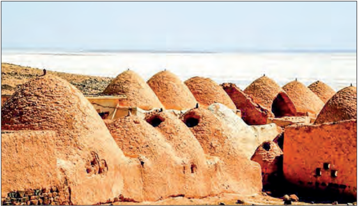
Also known as ‘beehive houses’, the conical adobe structures keep cool in the blazing desert sun, while their thick walls also retain warmth in the winter. PHOTO: AFP
