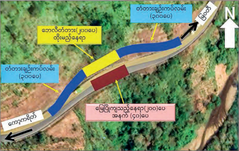
The aerial photo shows the construction site where a temporary bailey bridge is being built at the landslide-hit section of Asian Highway.
