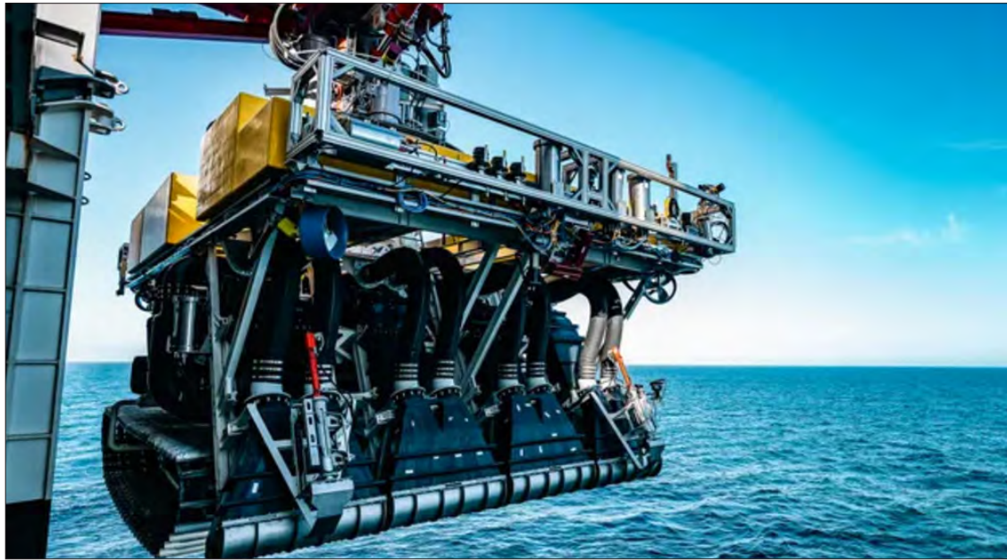
A pilot vehicle — called a nodule collector — used in deep-sea exploration is lowered into the water in trials conducted by mining group TMC. PHOTO: PIX FOR VISUAL PURPOSE/ RICHARD BARON/THE METALS COMPANY
