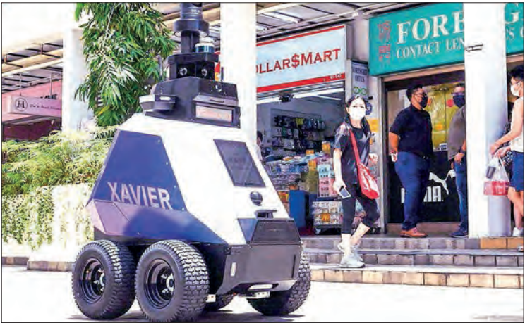
The robots are equipped with cameras, sensors, speakers, a display panel, blinkers and a siren. Singapore's Home Team Science and Technology Agency (HTX) roving robot has hit the streets of Toa Payoh Central as part of a trial to support public officers in enhancing public health and safety. PHOTO: AFP/FILE
