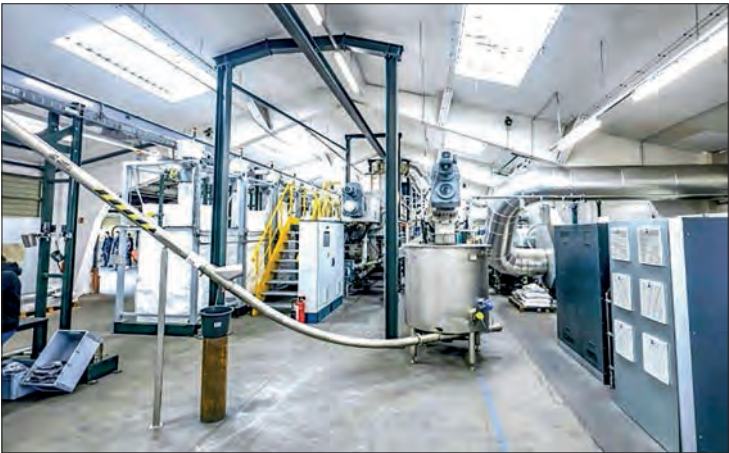
Biochar is produced by heating cocoa bean husks in an oxygen-free room to 600 degrees Celsius (1112 Fahrenheit). PHOTO: AFP
