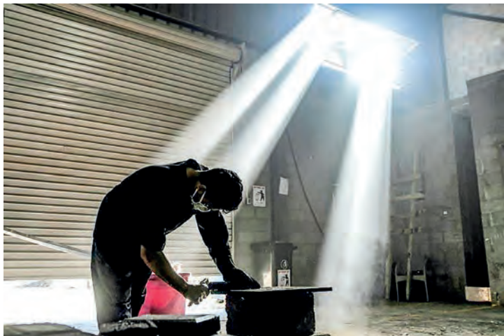
The plastic is shredded, liquefied and pressed into outdoor pavers for walkways and garages. PHOTO: AFP
