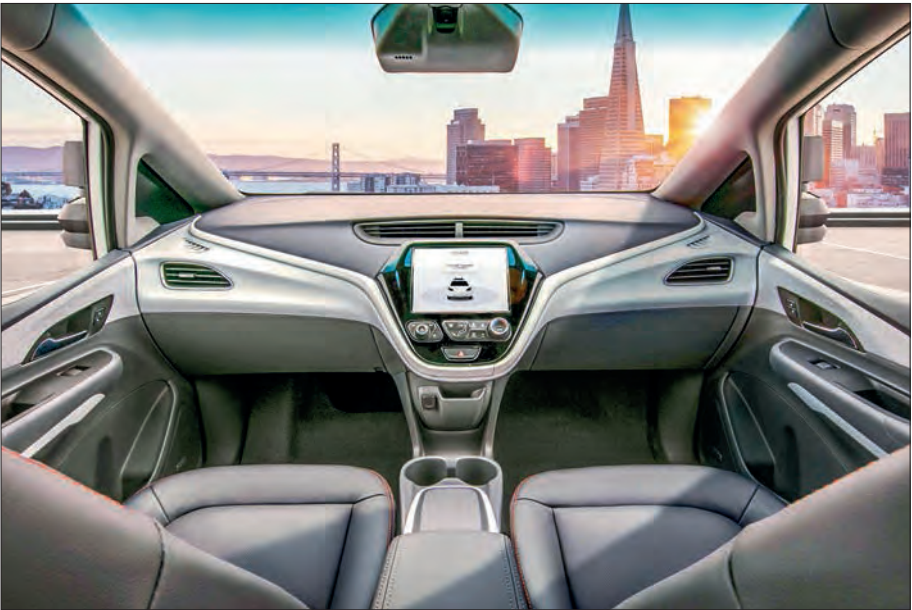
General Motor’s Cruise self-driving car is designed to operate on its own with no driver, steering wheel, pedals or other manual controls. PHOTO: GENERAL MOTORS/AFP/FILE
