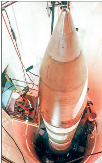
The Minuteman III was the first US Intercontinental Ballistic Missile (ICBM) that could deliver Multiple Independent Reentry Vehicles (MIRVs) to a target. A Minuteman III in silo undergoing maintenance. PHOTO: USAF/FILE
