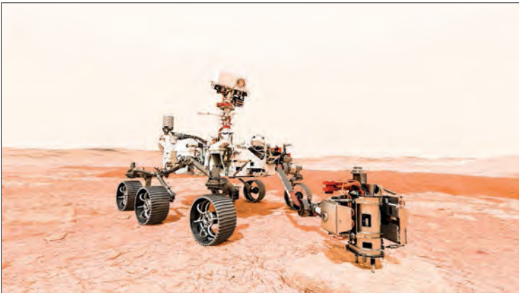
In this illustration, NASA's Mars 2020 rover uses its drill to core a rock sample on Mars. PHOTO: NASA/JPL-CALTECH/AFP
