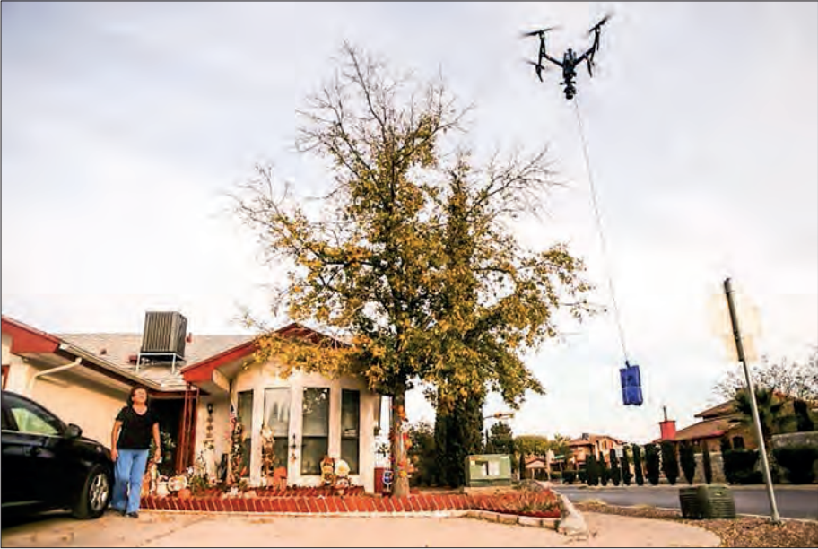
The drones can carry loads as heavy as five pounds (2.2 kilogrammes) in packages about the size of a large shoe box. PHOTO: AFP
