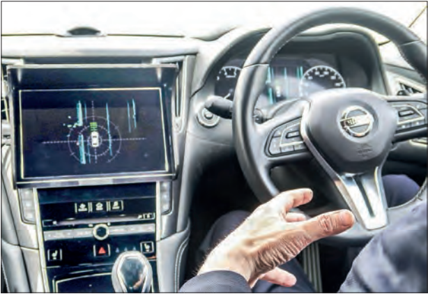
Photo taken in Yokosuka, Kanagawa Prefecture, on 18 April 2022, shows a monitor screen on a Nissan Motor Co test vehicle showing the position of objects in the vehicle's surroundings detected by sensors. PHOTO : KYODO ligence to warn drivers of imminent traffic hazards and help them avoid accidents caused by human error, aiming to equip its vehicles with the technology in the latter half of the 2020s. — Kyodo
