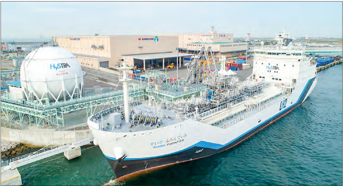
The Suiso Frontier is a world-first tanker built to transport hydrogen by sea. PHOTO: HESC PROJECT/AFP
