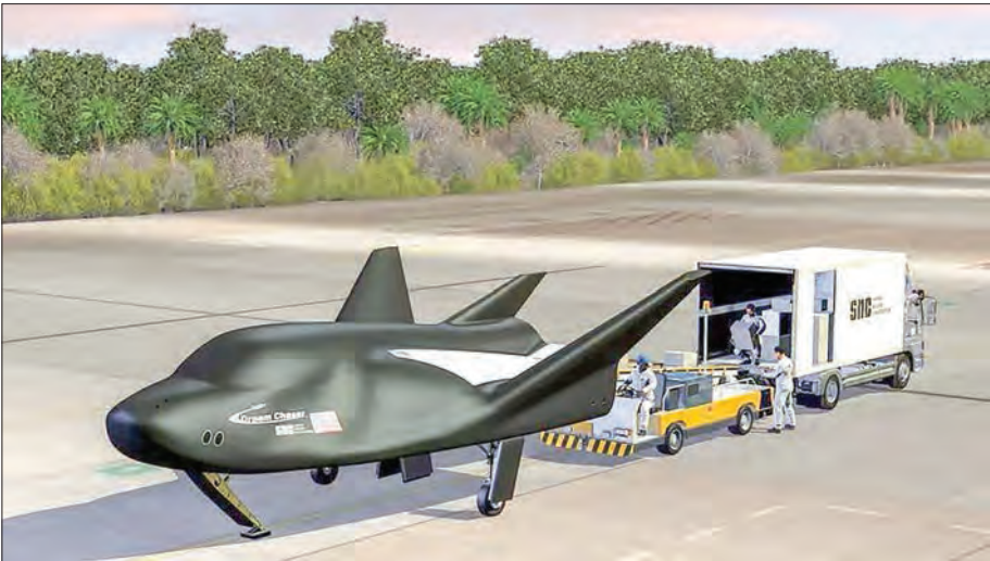
The Dream Chaser space plane is designed to return cargo to Earth by landing on a runway, allowing for rapid access. PHOTO: SIERRA NEVADA CORPORATION/AFP
