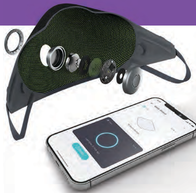
AirPop's Active+ mixes breathing sensors with air quality data. AirPop: The connected Halo sensor (just in the wearer's bottom-left) actively monitors user respiratory health stats and local air quality, providing feedback regarding breathing and mask performance through the companion app. PHOTO: AIRPOP/AFP
