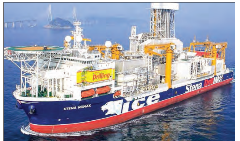
Stena IceMAX is the world's only 6th Generation Ice-Class Harsh Environment dual-activity dynamically positioned (DP3) drillship, capable of drilling in water depths up to 10,000ft.
