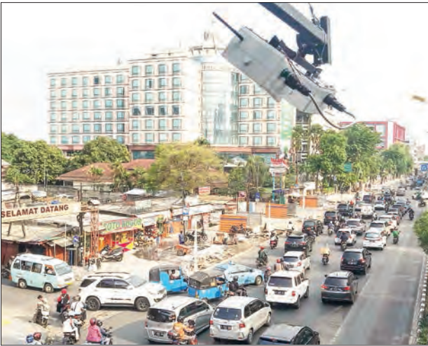
This photo shows a sensor unit for a device made by Murata Manufacturing Co. and installed in Jakarta to measure traffic data. PHOTO: KYODO
