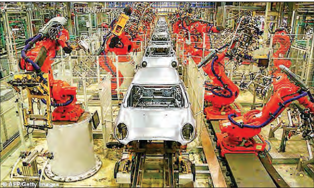
Robotic arms work on the bodyshells of Mini cars as they pass along a section of automated production line at the BMW Mini car production plant in Oxford in 2017. BMW, Peugeot PSA and Japan's Nissan have factories in the UK. FILE PHOTO: AFP
