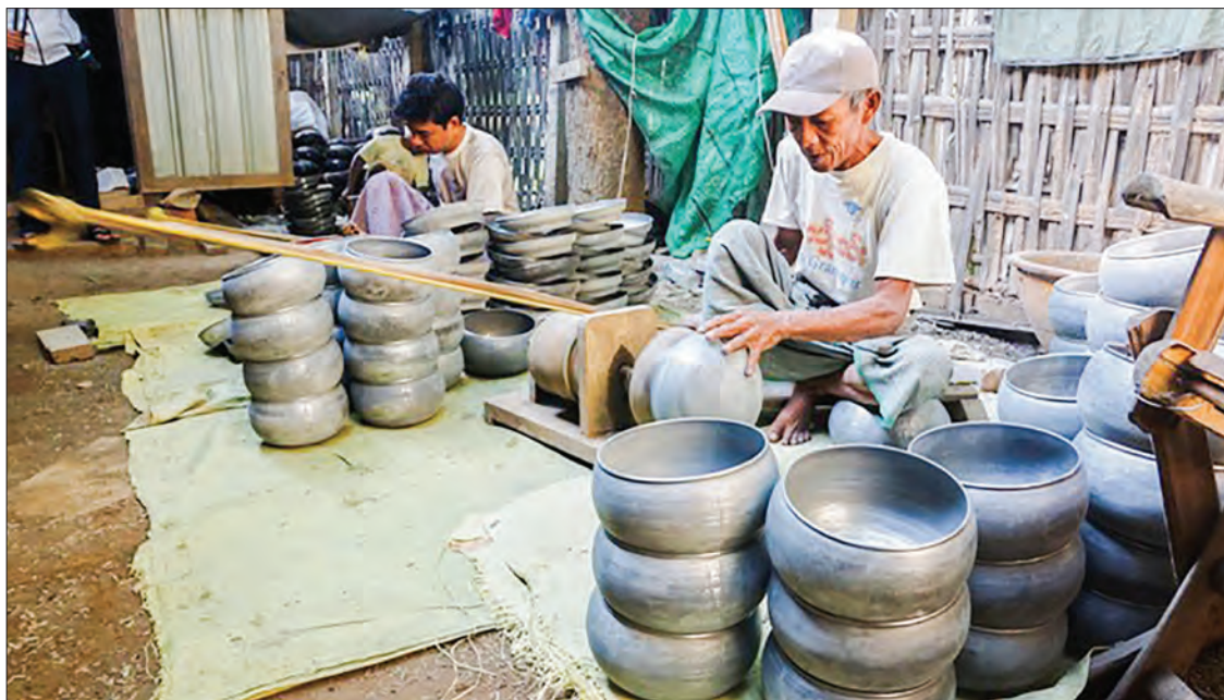
An artisan worker polishing an alms bowl to smooth the surface of the object. PHOTO: THAN ZAW MIN (IPRD)
