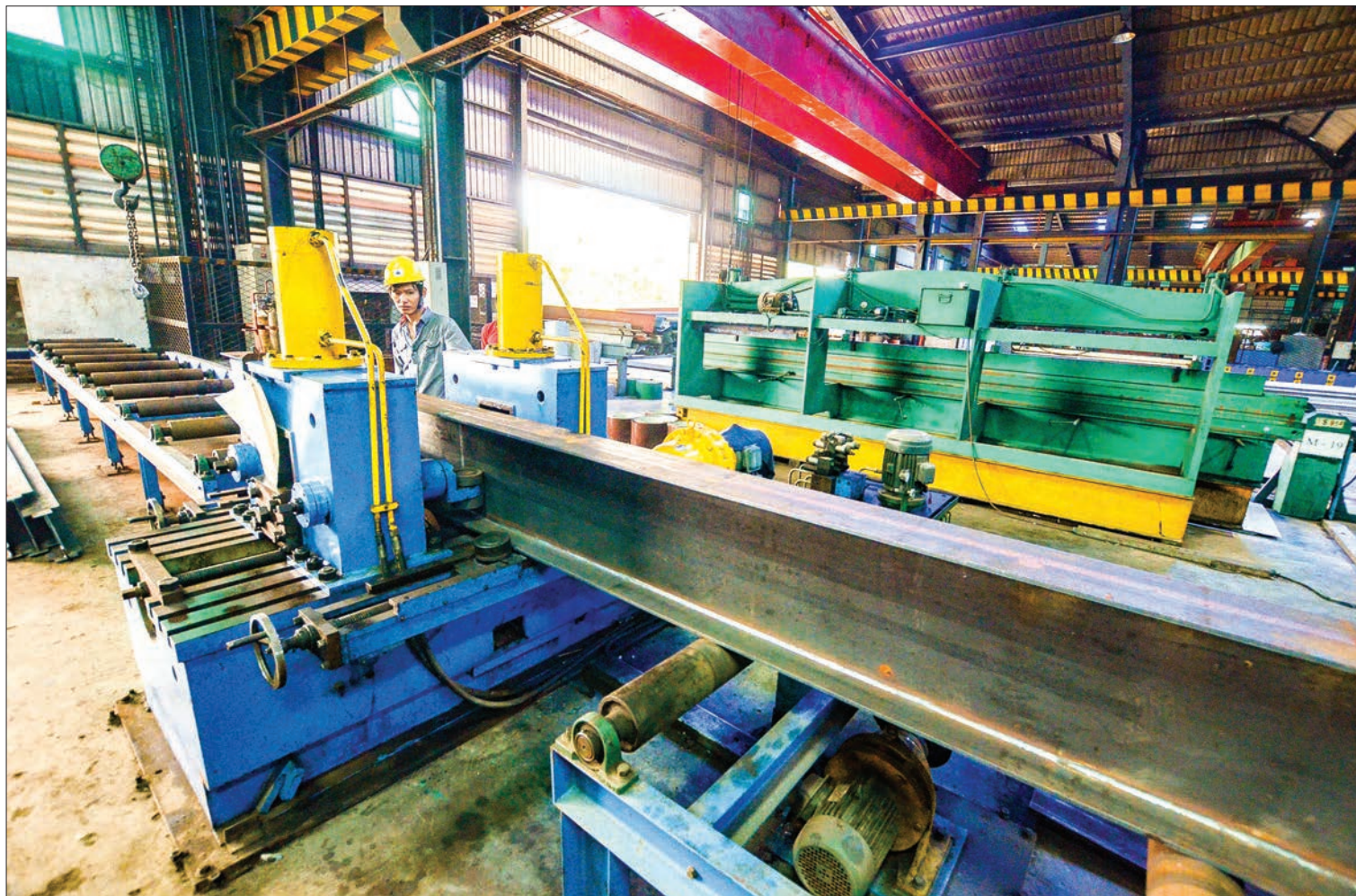
Hydraulic straightening machine in SMI. PHOTO: PHOE KHWAR
