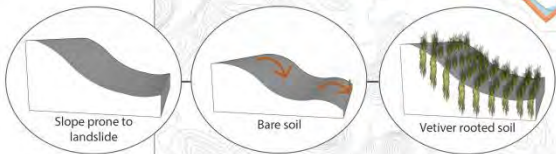
Slope treatment with vetiver grass:
